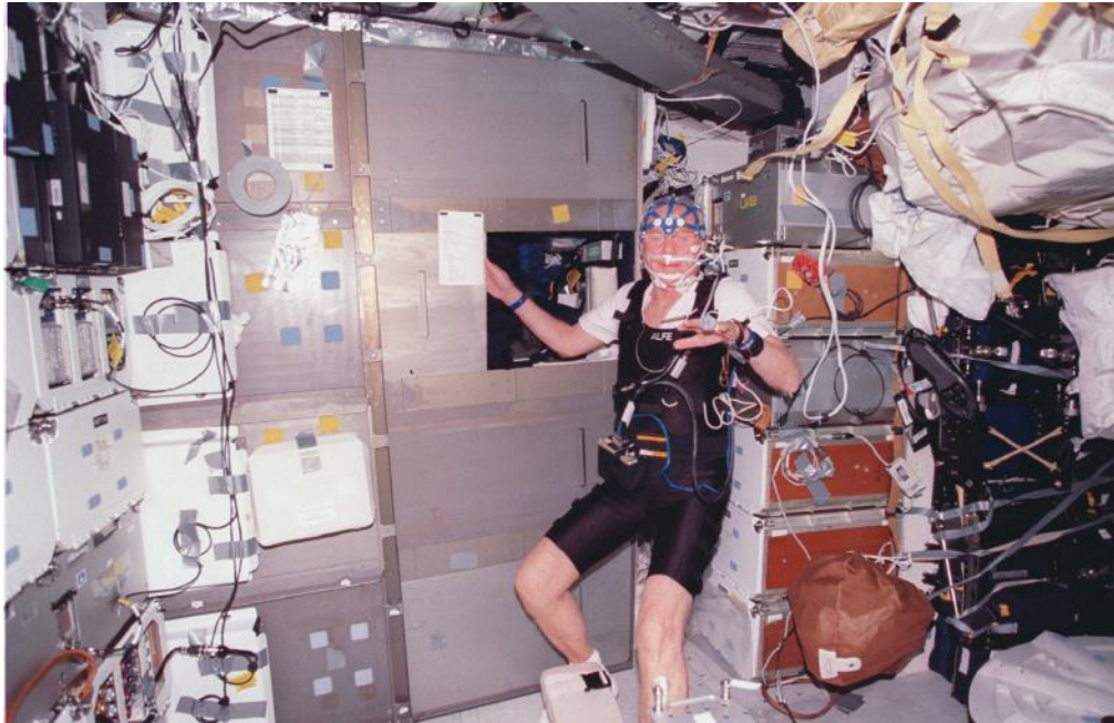
Figure 2.4: Astronaut John Glenn in Discovery’s mid-deck, ready to go to sleep. He is wearing all instrumentation of the sleep study, namely the sleep net (detailed photo below), and the custom-fitted two-piece lycra body suit, containing the rib cage and abdominal RIP sensors. On his finger one can see the pulse oximeter, and on the wrist a wrist activity monitor. All sensors are connected to the recorder, seen here on the astronaut’s belly, by a single cable. Behind are the 4 sleep compartments where subjects slept (Photo NASA). In his autobiography ([6]), John Glenn describes the night of this photo as follows: “Night four of the mission saw me (...) rigged up in our head nets and instrumented vest. The twenty-one leads from the apparatus fed into boxes we wore on our waists, where the information was recorded for later analysis. We repeated everything the next night. (...) Sleeping with the elaborate head net and vest turned out to be easier on orbit than on the ground, where the electrode leads were uncomfortable. Imagine sleeping with a dozen buttons over half an inch thick stuck on your head that you feel every time you roll over. Weightlessness removed the irritating pressure. (...) On nights 7 and 8 (...) I put the sleep nets and vests on again for two more sets of readings.”
